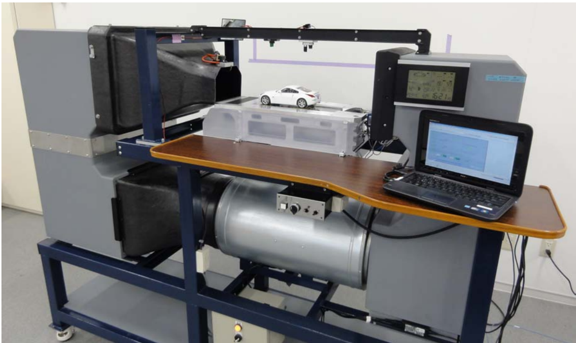
Photo 1: Super Small Wind tunnel
