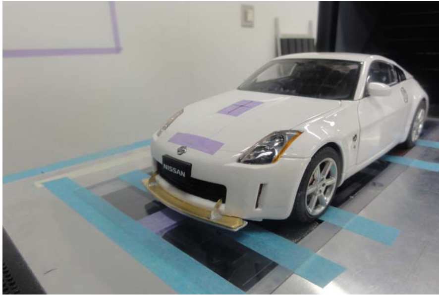
Photo 3: Full scale Comparison Setup Super Small Tunnel (SST)
